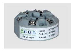
The head-mounted version of the Temperature Transmitter Models Fr Block for RTD Pt-100 sensor input and Thermocouple input, converts a standard temperature sensor input signal into a 4 to 20 mA DC current loop signal with excellent linearity and load driving capability.
