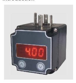
The LPI-PT is a microprocessor controlled loop powered display for any  $4 \sim 20$  mA standard signal. It does not require its own separate voltage source as it is supplied directly from the measuring current loop.
